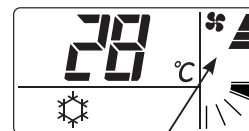
The fan speed is set to “High” in the cooling operation.
